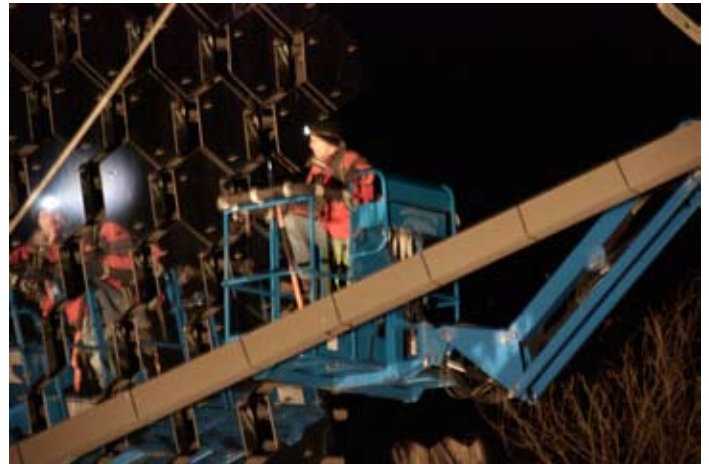
Dr. Karlsson aligns one of the over one thousand mirrors of the VERITAS telescope array using a laser alignment tool, a cherry picker and a wrench. Image Credit: Larry Ciupik.
