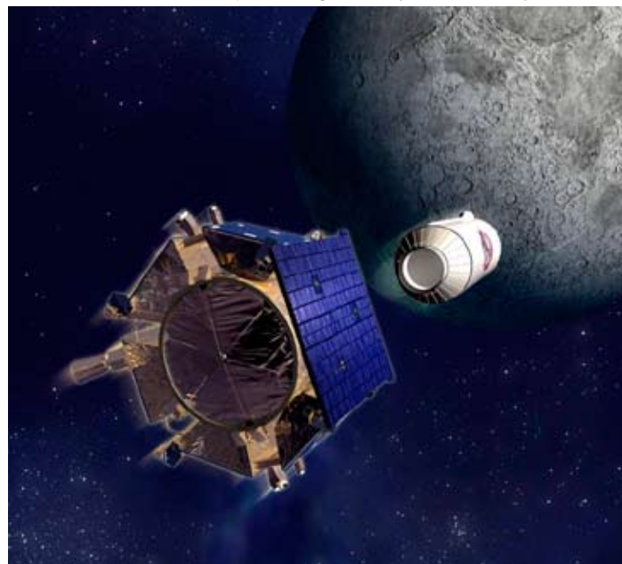
Atlas Centaur upper stage separates from the LCROSS spacecraft bus on its approach to the Moon. Both the upper stage and the spacecraft will impact the Moon on October 9, 2009. Image credit: NASA
