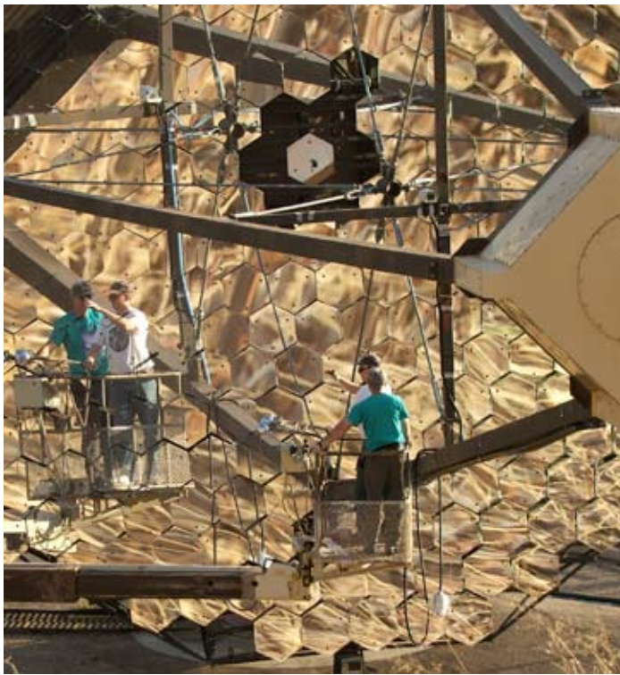
Adler Astronomer Larry Ciupik works on the T1 VERITAS telescope with Dirk Pandel from University of Iowa to install video cameras for monitoring the position of the telescope. Image credit: David Steele
