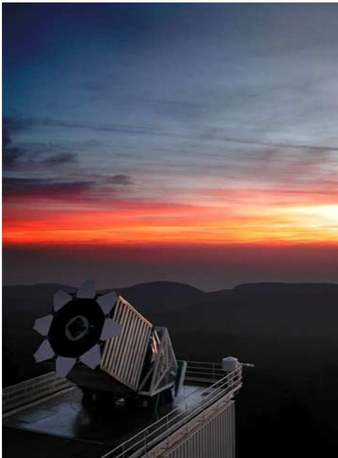
The 2.5-meter telescope at Apache Point Observatory. Specially built for the Sloan Digital Sky Survey, the 2.5-meter has numerous innovations such as a roll-off enclosure and advanced wind-shedding light baffles. Image credit: José Francisco Salgado
