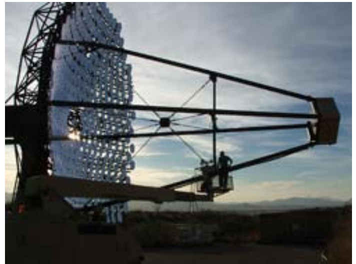
An astronomer inspects the lower quadrupod arm of T1, one of four telescopes of the VERITAS gamma-ray observatory located at Fred Lawrence Whipple Observatory in Arizona. Each telescope has 350 mirror segments forming a primary reflector 12 meters in diameter. Image credit: David Steele
